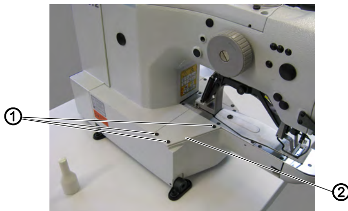
Fig. 5: Removing and fitting the left-hand side cover
