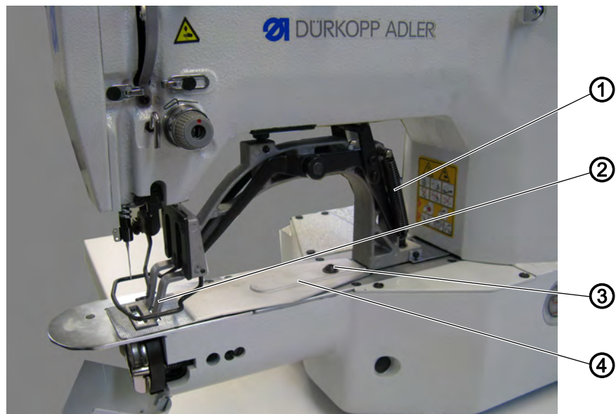
Fig. 8: Removing and inserting the throat plate (1)
